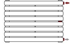
Connection with couplings welded laterally with diaphragm
