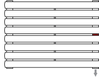
Connection on the right manifold with diaphragm
