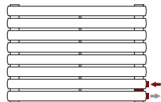
Connection with welded couplings, 50 mm pitch, on the left side
